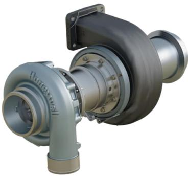
Turbo lag affects drivability and Real Driving Emissions. It is addressed, but not completely eliminated, with known compromises in turbo matching and design, that are detrimental to the engine fuel efficiency. Turbo lag is due to a temporary lack of turbine power, caused by too low enthalpy in the exhaust gas, at the begin of load steps.
